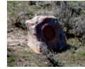
Noise was broadcast at 70dB SPL at 16 meters from 4 rock-shaped speakers on treatment leks
